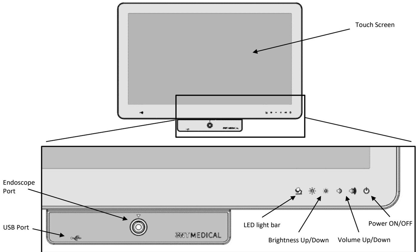
**Figure 1 - Console Front Panel**
